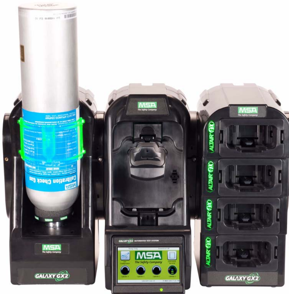
Fig. 1 The GALAXY GX2 Automated Test System
