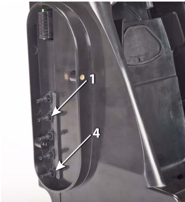
Fig. 17 Gas inlets on the Test Stand
