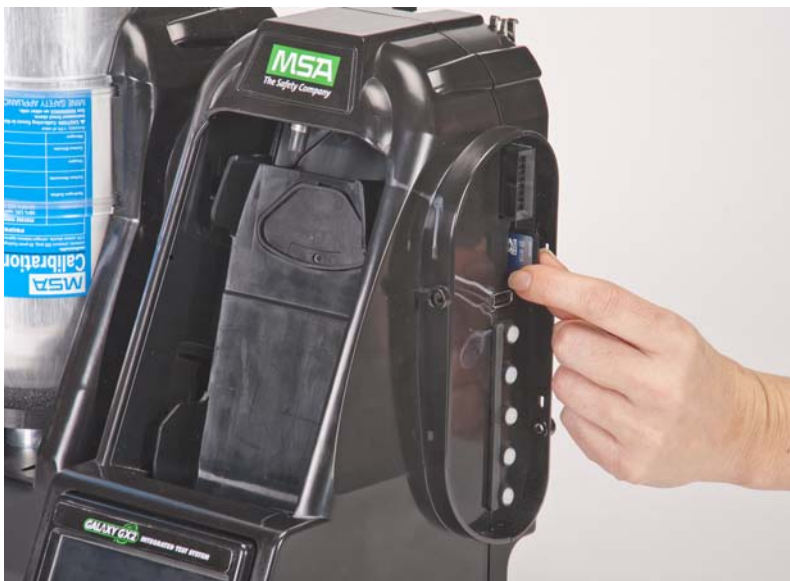
Fig. 13 SD or SDHC Memory Card Installation
