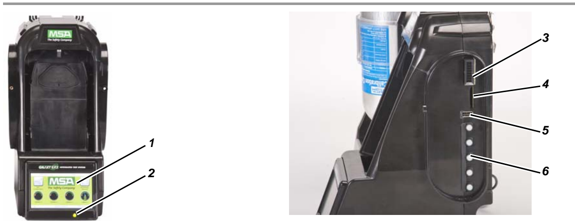
Fig. 3 Test Stand Physical Features
