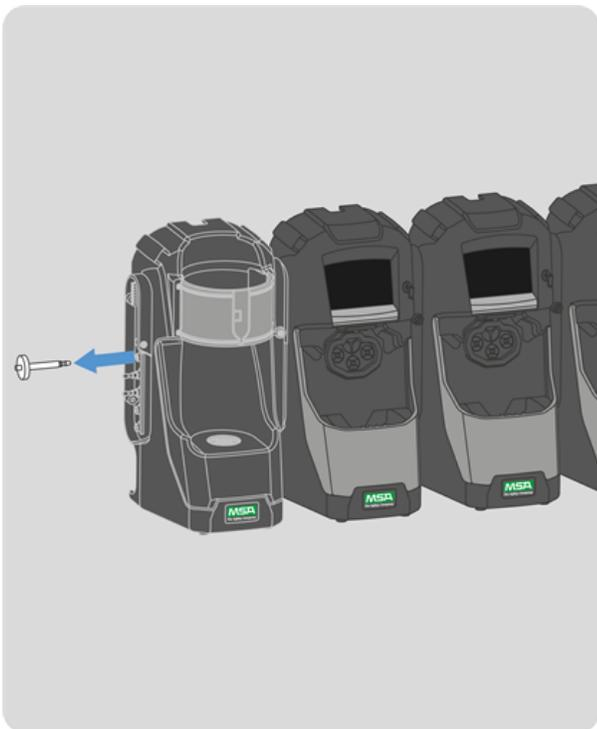
1. Remove the filter and tubing from the barb fitting in the fresh air port on the left side of the farthest left unit.
