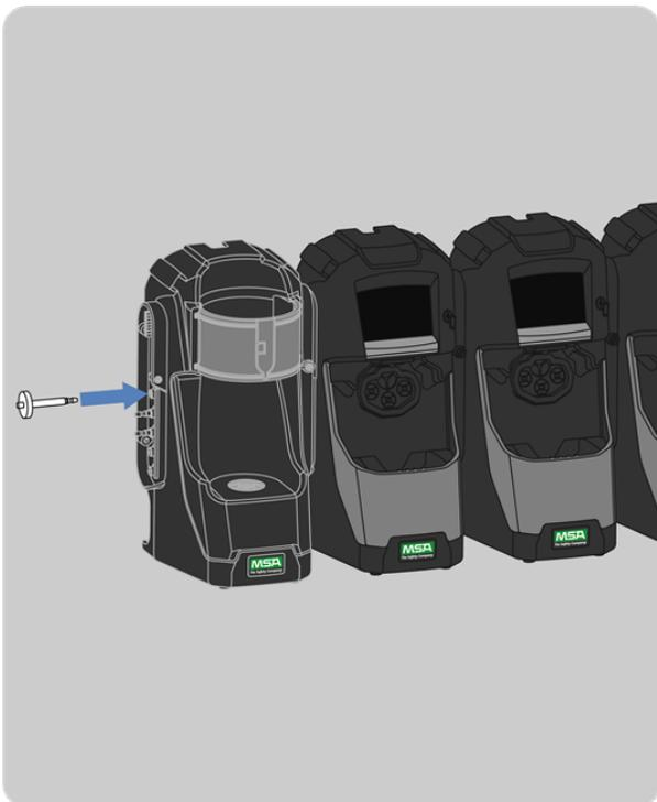
3. Insert the new filter and tube onto the same barb fitting of the fresh air port.
