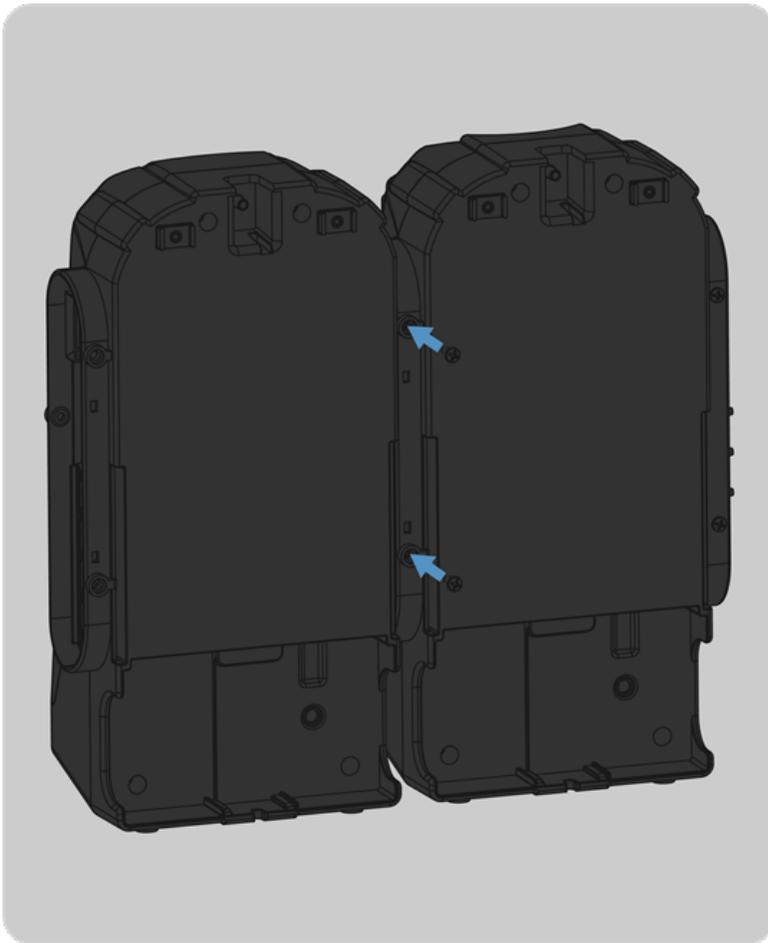
10. Screw the Cylinder Holders together using the supplied screws.
