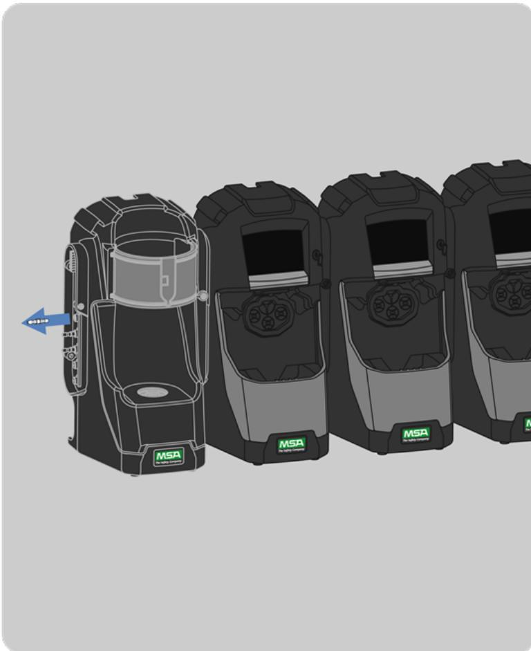
11. Remove the top barbed connector from the left most cylinder holder.
