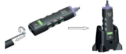
Figure 2 Charging Device in Charging Cradle
