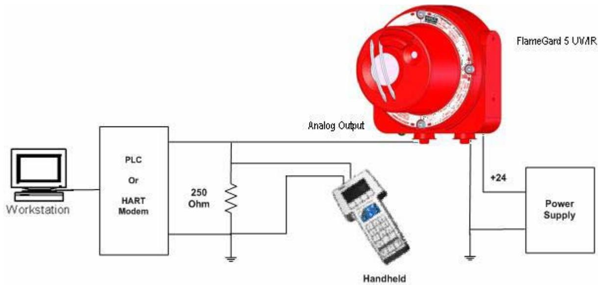
**Figure 1 : Connecting a PC to a HART device**
