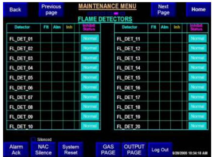
Figure 11: Secondary Fire Alarm Maintenance Screen
