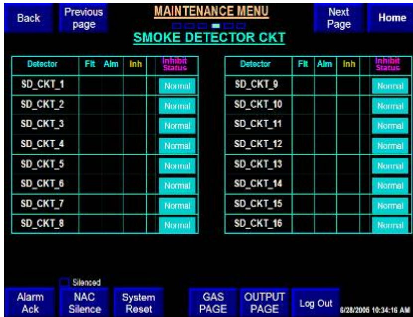
Figure 64: Fire Alarm Maintenance Screen
